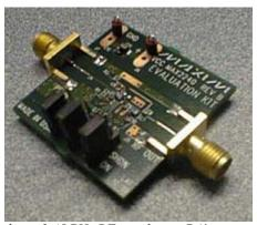
Objective: To improve the low voltage 2.45GHz RF non-linear PA's output matching network using mainly lumped surface mount components.
